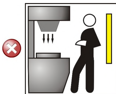
Figure 7: Wrong light curtain positioning
