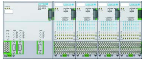
Abb. 3: MVB Buscoupler with I/O Modules
