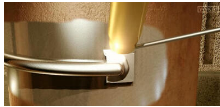
Fixed connection (compression fitting) to the furnace
