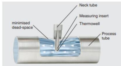
The patented hygienic design of the TW61 flow-through housing enables minimised, invasive temperature measurement and a flexible mounting position through self-draining.
