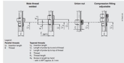
Fig. with parallel thread, for tapered thread see "Process connection"
