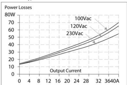
Fig. 12-1 Efficiency vs. output current at 24V, typ.
