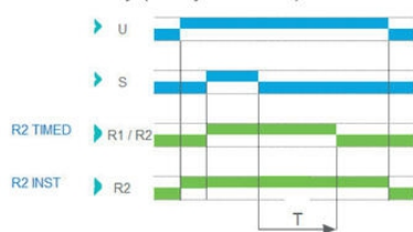
Function C - Off-Delay (Delay on break)
