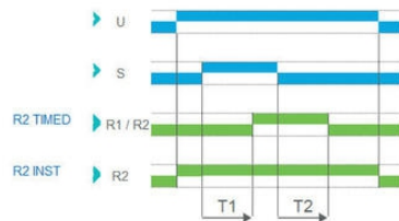
Function Ac - On/Off Delay (Delay on make/break)
