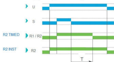
Function C - Off-Delay (Delay on break)
