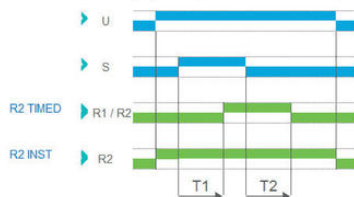
Function Ac - On/Off Delay (Delay on make/break)
